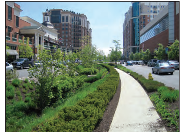
Rain gardens and other bioretention techniques can be installed in small spaces within urban environments.
